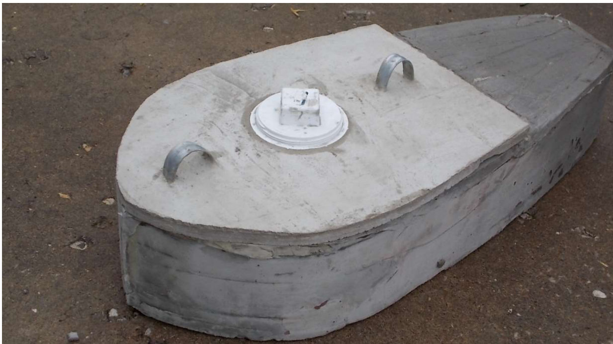
Figure 1. The original design for the Hellbender nest box, fresh from the mold, was created using a multipiece wooden mold. The lid is molded separately, and fits into the top of the nestbox.
