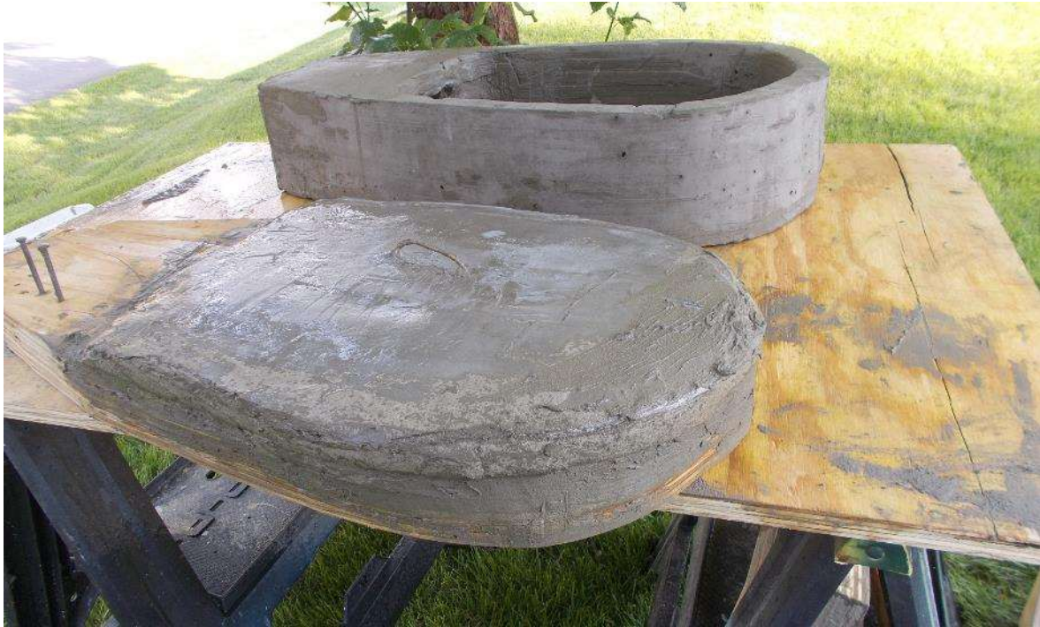
Figure 1. The original design for the Hellbender nest box, fresh from the mold, was created using a multipiece wooden mold. The lid is molded separately, and fits into the top of the nestbox.
