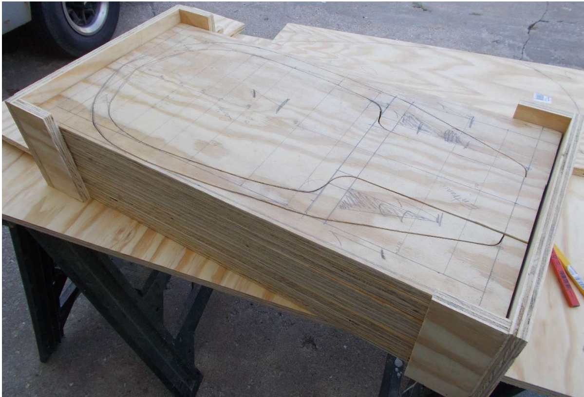
Figure 3. The outer securing form is shown with the inner shaping forms stacked inside.
