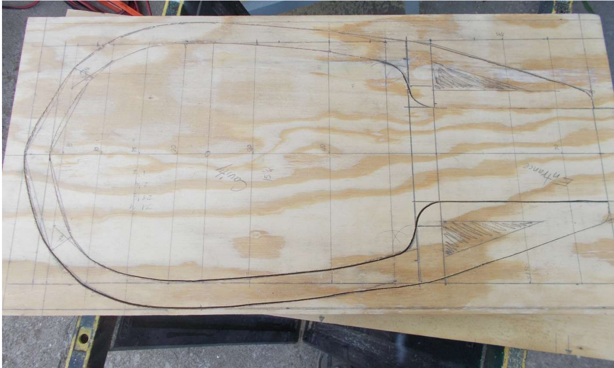
Figure 5. Cutting along the lines yields three pieces: the inner shaping mold, the outer shaping mold and the blank area in between where the concrete will cure.
